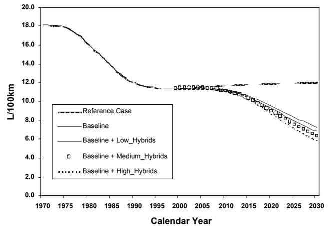
Figure 8: Average light-duty vehicle fuel consumption for various technology scenarios.
