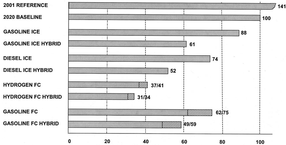
Figure 1: Relative on-board consumption of fuel energy for vehicle technology combinations. MJ(LHV)/km expressed as percentage of baseline vehicle fuel use. All vehicles (except 2001 reference and 2020 baseline) are advanced 2020 designs. Driving cycle assumed is combined Federal cycles (55% urban, 45% highway). Hatched areas for fuel cells show increase in energy use in integrated total system which requires real-world compromises in performance of individual system components.
