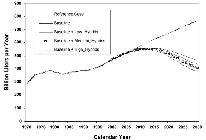
Figure 7: Light-duty fleet fuel use for various technology scenarios.
