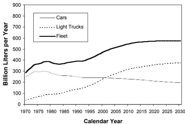
Fig. 10: Stabilization in light-duty vehicle fleet fuel use due to a steady 1.3% annual decrease in average new vehicle fuel consumption.
