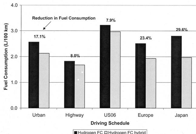
Figure 3 shows the results for the advanced fuel cell and fuel cell hybrid vehicles. The trends are similar, but the percentage hybrid fuel consumption benefits are significantly lower. Since the fuel cell is relatively more efficient at lighter loads, whereas the ICE exhibits the reverse trend, this part of the hybrid benefit (shifting the “engine” to higher loads) is much reduced.
