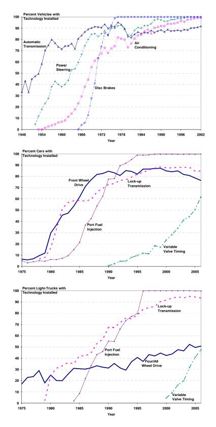
**Figure 47** Technology deployment in new vehicles, 1948–2006 [Ward's 2003; Heavenrich 2006]
