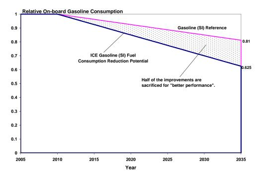
**Figure 22** Average U.S. car relative onboard gasoline-equivalent fuel consumption at 50% ERFC
