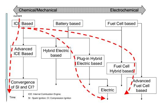
Figure 8 Possible propulsion system pathways
