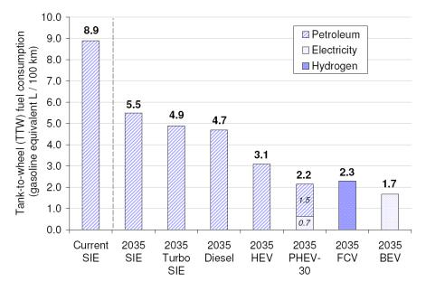
(a) Tank-to-wheel gasoline-equivalent (GE) fuel consumption.
