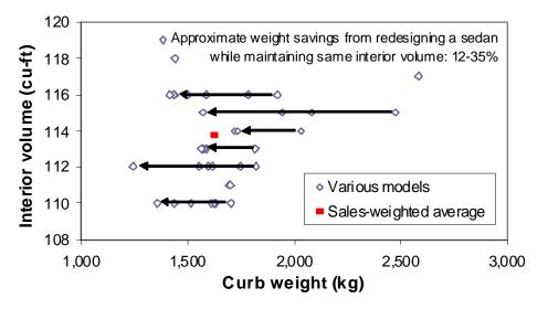
**Figure 16** Potential weight savings from redesigning model year 2007/2008 midsize sedans while maintaining same interior volume
