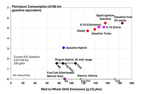
Figure 44 Fuel consumption and well-to-wheel GHG emissions for future (2035) cars
