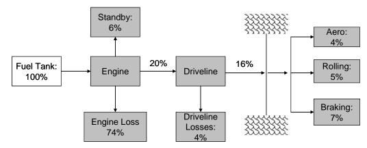
Figure 9 Representative vehicle energy flows in an urban driving cycle
