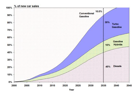
Figure 52 Turbocharged ICE Future Scenario
