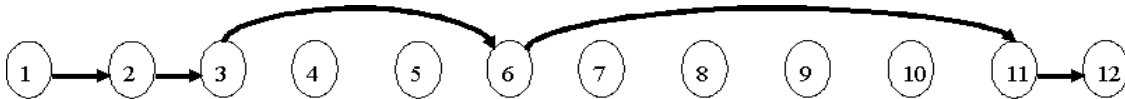
Figure 3. Let tour T = (1, 2, 3, 4, 5, 6, 7, 8, 9, 10, 11, 1) . After applying the CI 2-opt moves implied by the path 1 - 2 - 3 - 6 - 11 - 12 tour T = (1, 2, 3, 5, 4, 6, 10, 9, 8, 7, 11, 1) is obtained.
