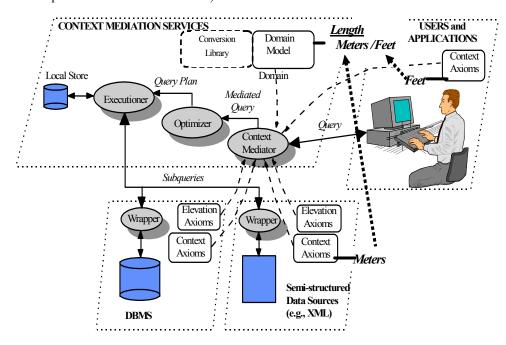
Fig 5. The Architecture of the Context Interchange System
