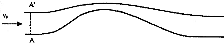
Figure 9P.2 Flow in a Gap Between Two Curved Surfaces
