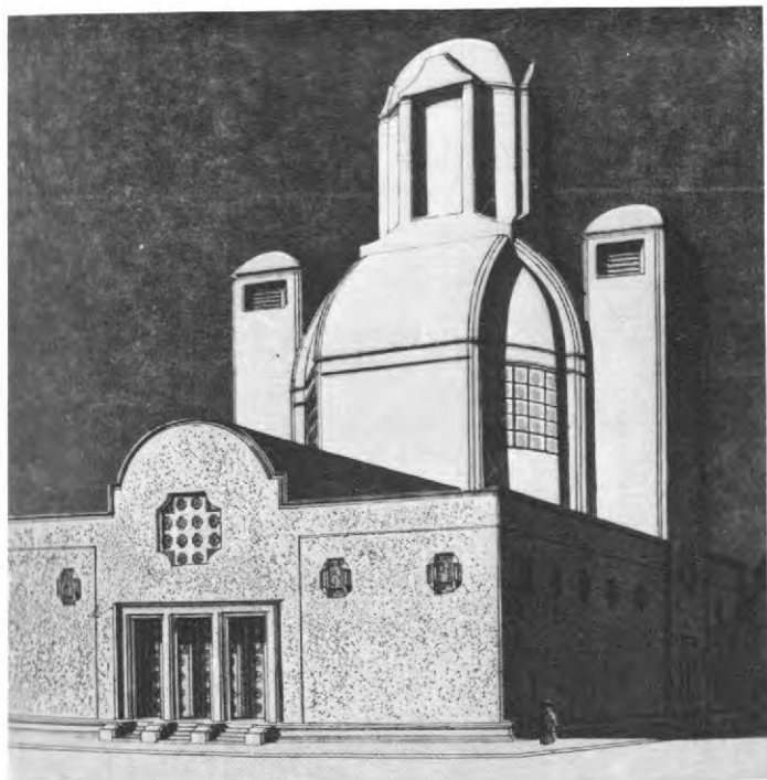
8 Project for a church. Christian Bayer, pub. 1909. Perspective. Designed according to a method advocated by J.L.M. Lauweriks in which the same differentiated grid underlay the plan, sections, and elevations.
