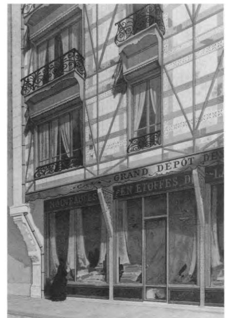
9. Viollet-le-Duc, street building with a modern iron frame and ceramic infill. ( Entréens sur l'architecture , atlas [Paris: A. Morel et Cie, 1864], plate 36.)
