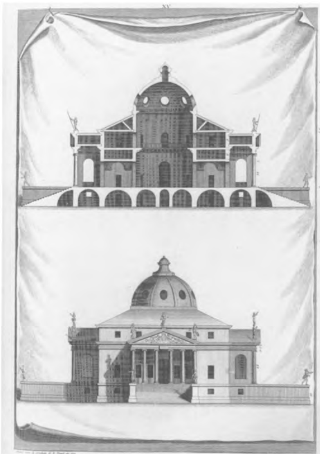
FIG. 10: Andrea Palladio, Vicenza, Villa Rotonda. Section and elevation from Giacomo Leoni’s edition of Palladio (London, 1715–16).
