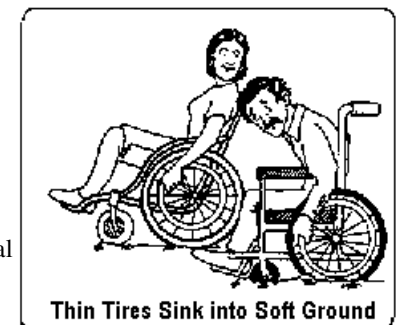
Thin Tires Sink into Soft Ground Drawing from "Independence Through Mobility" by Ralf Hotchkiss.
