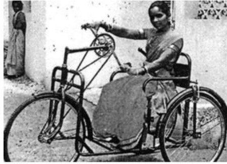
India. Hand-crank powers the front wheel. Good for flat paved roads; poor traction on hills and sand.
