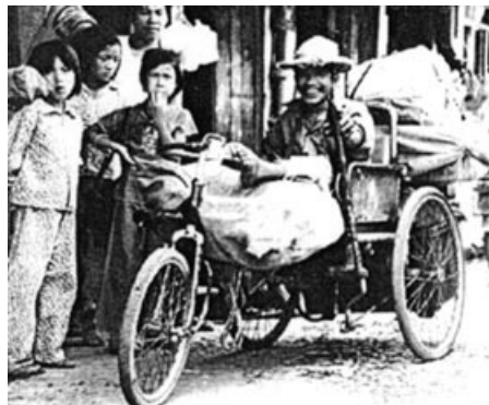
Thailand. A hand-pump powers one rear wheel. Steers with foot. Heavy duty for hauling cargo.
