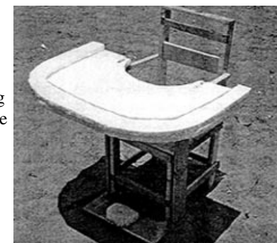
Participants made a child's seat from scraps of wood and foam plastic. They put a raised border on the table to help keep toys from falling off.
