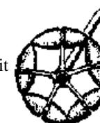
Ralf's "Ezekiel wheel." The small rollers roll sideways. The main wheel rolls forward. This gives a multi-directional caster effect, without swiveling.
