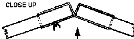
Cord laced in figure-8 for easy bending, as seen in this cross section.
