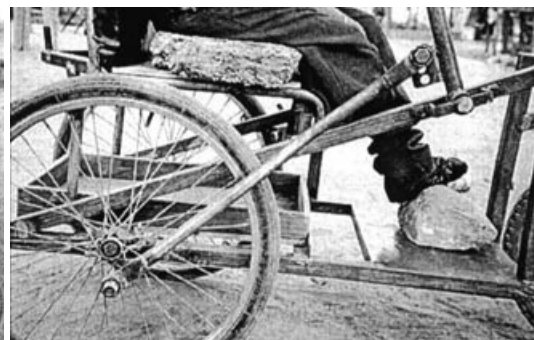
The hand-powered lever is attached to an arm welded to the hub and a bracket welded to the frame. It works like the drive mechanism of a railroad train.
