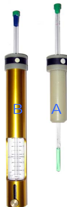
Figure 2: Spinner and Tube (A) Spinner and tube inside a depth gauge (B)
