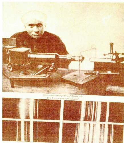
Figure 2: CV Raman with spectrograph, Raman tube and first Raman spectra photographed.
