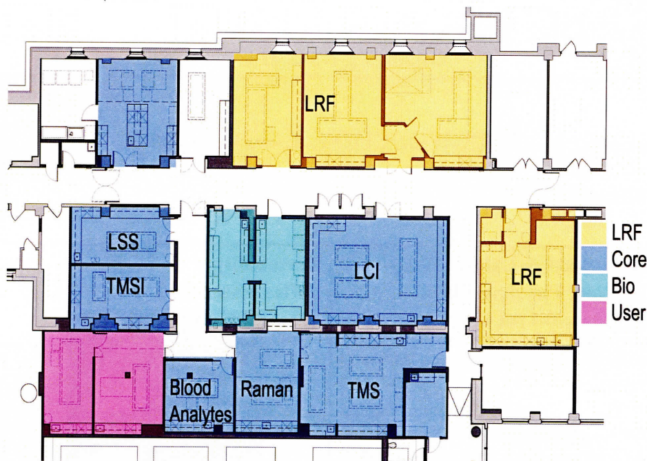
Floor plan for the renovated Spectroscopy Laboratory, ground floor of Bldg. 6. Researchers offices, probe facility and administrative offices are located on the second floor (not shown). Individual laboratories correspond to research programs of the LBRC (blue), LRF (yellow), wet chemistry and cell culture and facilities (green), and outside user facilities (purple).
