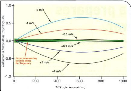
Changing the velocity of a Chinese warhead along its polar trajectory by very slight amounts (on the order of lm/s out of 7,000m/s total speed) produces measurably different trajectories. This graph shows the differences in range as a function of time after burnout for trajectories differing by these small amounts. These differences get significantly greater than the errors associated with measuring the warhead's position using China's navigational satellites, which is shown in green.
