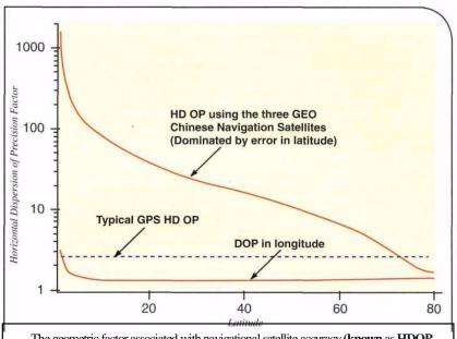
The geometric factor associated with navigational satellite accuracy (**known** as **HDOP**, for Horizontal Dilution of Precision) is shown here as a function of user latitude for the Chinese navigational satellite system. To determine the actual error, this geometric factor should be multiplied by an error determined by the electronics, atmospheric effects etc, which for GPS systems amounts to about 3m.
