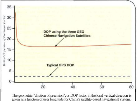
The geometric "dilution of precision", or DOP factor in the local vertical direction is given as a function of user longitude for China's satellite-based navigational system. To determine the actual error, this geometric factor should be multiplied by an error determined by the electronics, atmospheric effects etc, which for GPS systems amounts to about 3m.
