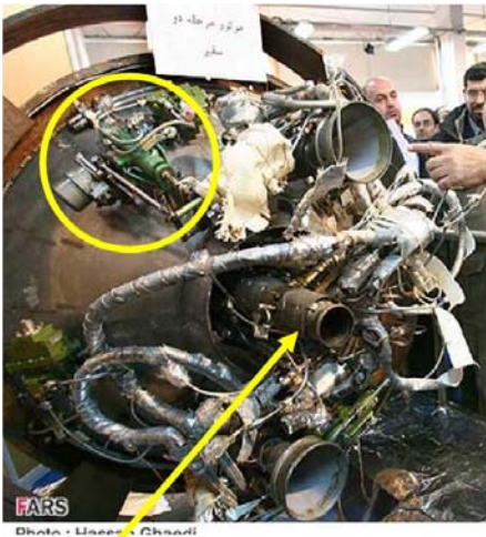
Exhaust manifold to central turbopump
