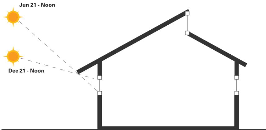
**Fig 1.8 Section of a building with sun positions at noon on equinox days**
