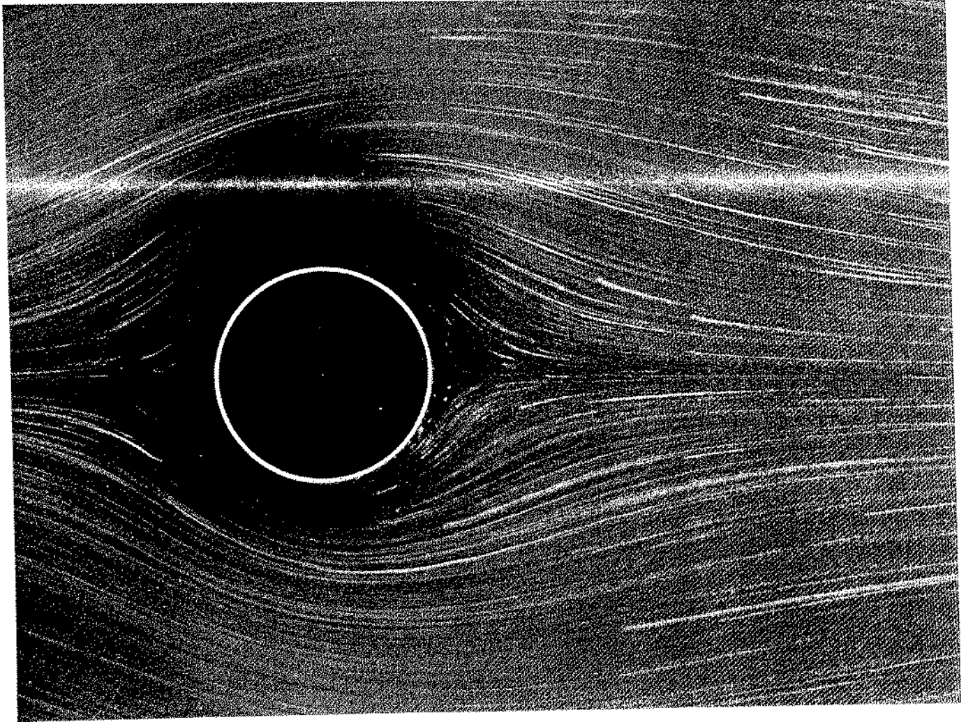
24. Circular cylinder at R=1.54 . At this Reynolds number the streamline pattern has clearly lost the fore-and-aft symmetry of figure 6. However, the flow has not yet separated at the rear. That begins at about R=5 ,
