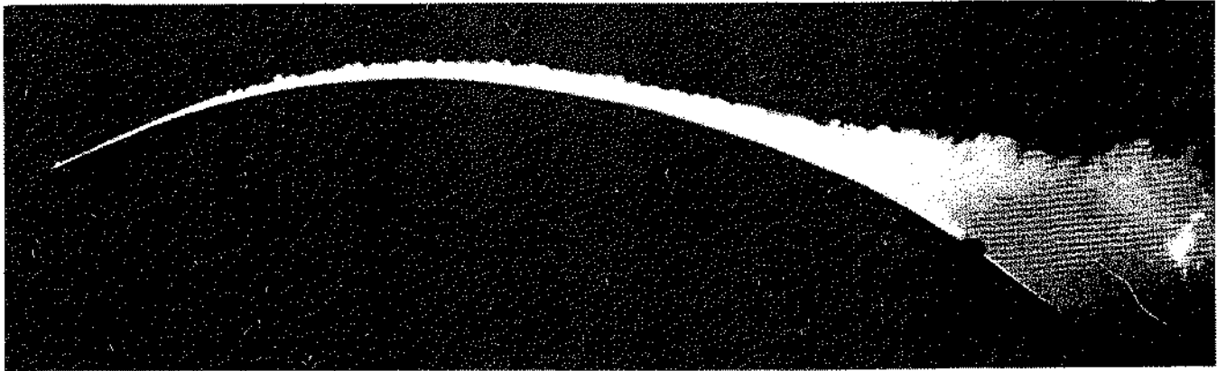
156. Comparison of laminar and turbulent boundary layers. The laminar boundary layer in the upper photograph separates from the crest of a convex surface (cf. figure 38), whereas the turbulent layer in the second
