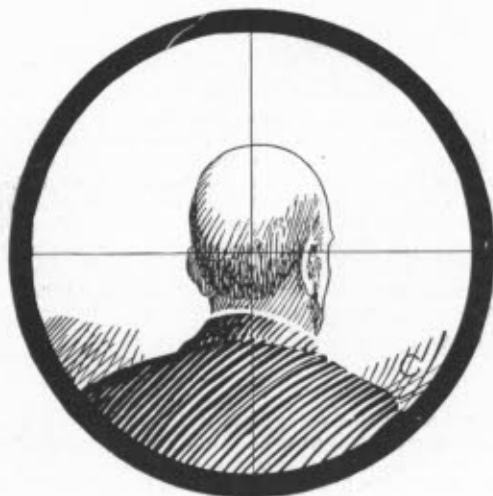
The "Cross hairs" as they appear in the modern telescope.
