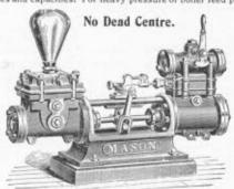
Outside Valve Adjustment. Seamless Copper Air Chambers. Tobin Bronze Piston Rods, Long Stroke.
