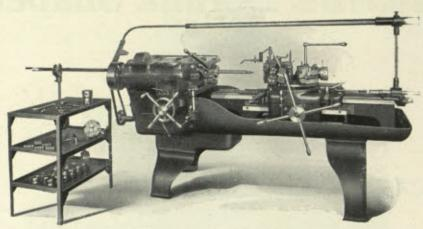
21/4 x 24 in. Set Up for Bar Work
