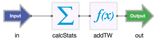
Figure 13. This is the same implementation event flow that is used to calculate every time-windowed feature.
