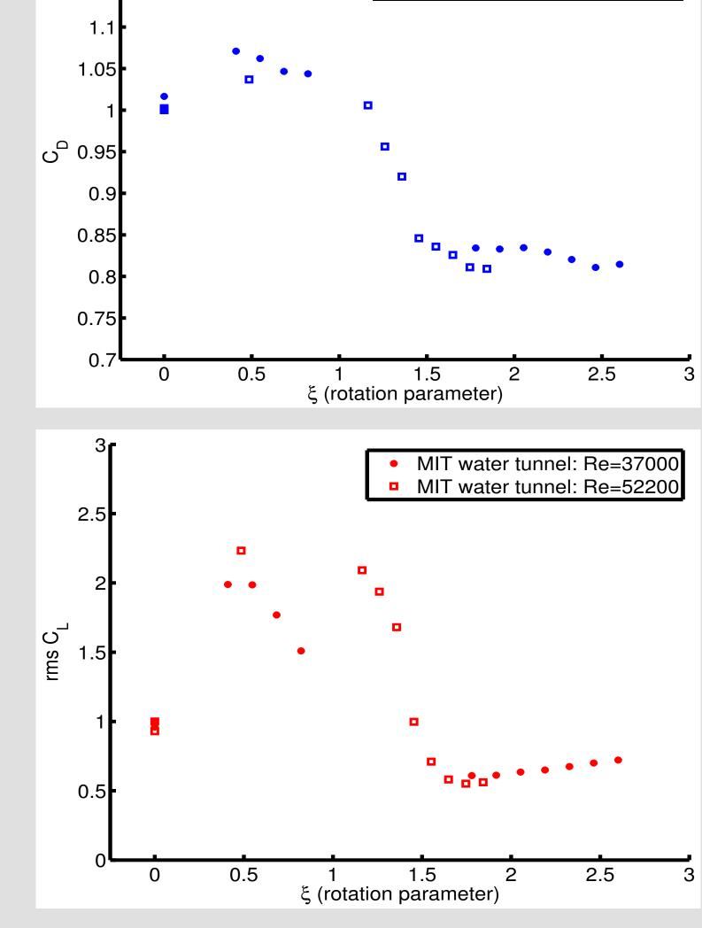
**Top:** Drag force normalized by drag measured with zero control effort. Bottom: RMS lift force fluctuations normalized by rms lift fluctuations with zero control effort.
