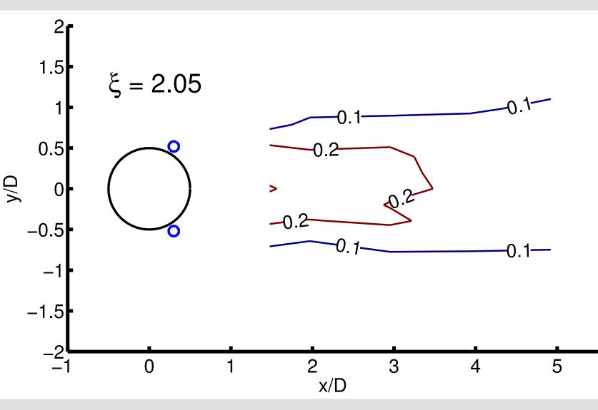
Contours of the root-mean-square transverse velocity component, normalized by the free stream velocity, are plotted on top of the mean velocity field variation from the free stream (black arrows). The free stream is directed from left to right. **Top:** The control cylinders (blue) are not rotating. Bottom: The control cylinders rotate such that the cylinder surface moves at a speed twice that of the free stream flow.
