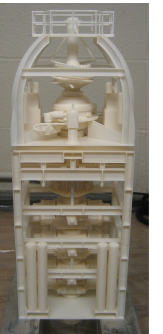
Fig.1 3D-printed, scaled model of the BOP
