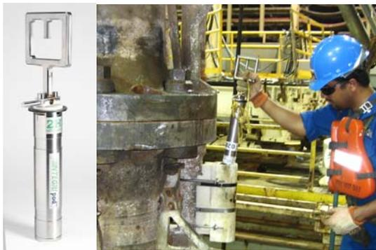
**Figure 4 – INTEGRIpod Motion Logger**
