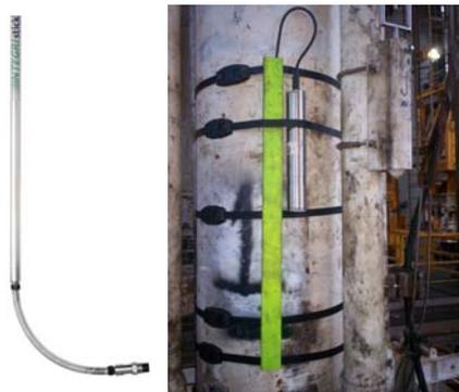
**Figure 5 – INTEGRIstick Strain Sensor**
