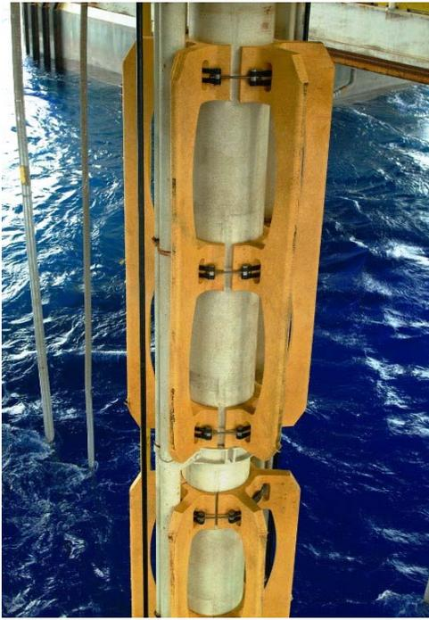
**Figure 2 – Lankhorst Fins on Drilling Riser**
