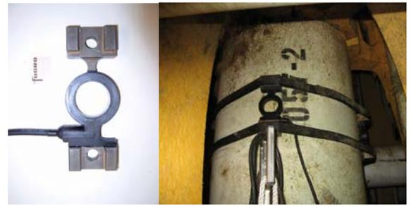
**Figure 6 – Fugro Proving Ring**
