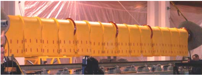
Figure 11: AIMS Dual Fin Splitter fairing Installed on Dynamometer
