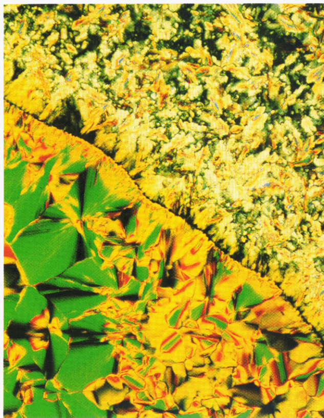
Figure 2. Photograph of a contact preparation showing the lack of miscibility of the O_h phase of 3 , N = 12 (bottom) with a D_{hd} phase of a square-planar copper diketone complex (top) viewed with a polarizing microscope at 90 °C (polarizers oriented vertical and horizontal).
