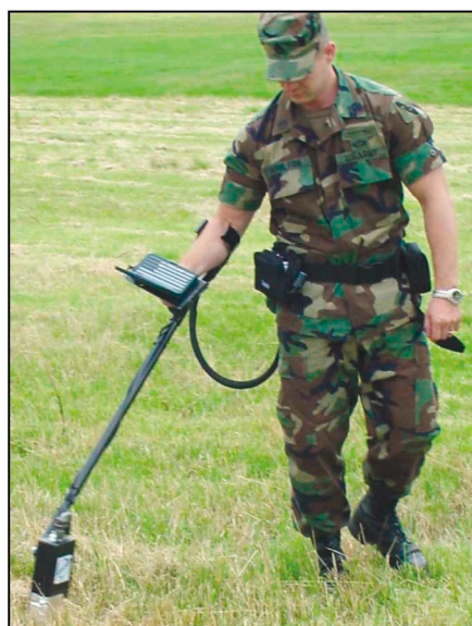
Figure 2. Land-mine detector, based on self-amplifying polymers, undergoing field tests. This prototype, the FIDO 4A, is capable of detecting femtograms ( 10^{-15} g) of TNT and has undergone extensive field testing at Fort Leonard Wood, Mo., and the Yuma Proving Ground, Ariz., as well as in Croatia. (Photograph courtesy of Nomadics Inc.)
