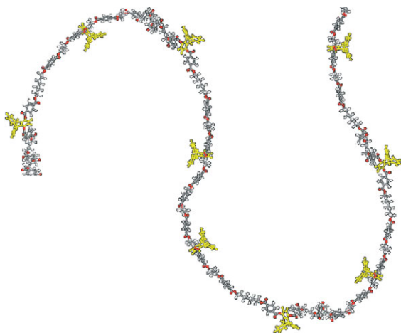
Figure 2. Schematic of pendant units with IMFV generating a polymer-chain contour resembling "molecular barbed wire".
