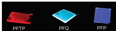
Figure 4. Fluorescent images of thin films of PFTP , PFQ , and PFP under UV irradiation (365 nm).
