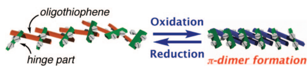
Figure 1. Schematic illustration of a molecular actuation triggered by a \pi -dimer formation of oligothiophene moieties connected with electronically inactive hinge parts.
