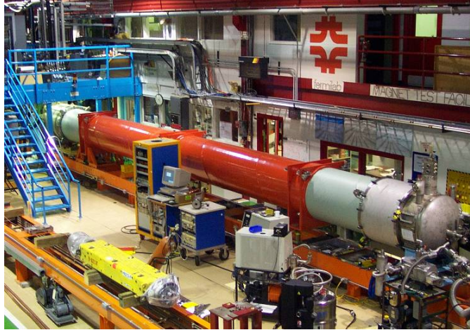
Figure 3.18: Cross-section of the MQXB low- \beta quadrupole (left) and Q2 quadrupole on test in FNAL (right).
