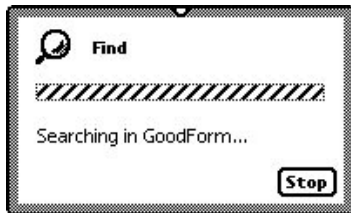
Figure 17-6 Progress slip with barber pole gauge
