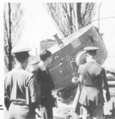
4. When searchlight has been pointed from control station, the beam is switched on. Only a little movement is generally necessary to find the plane. Thus the position of the battery is not disclosed until last minute.
