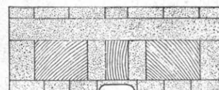
Cross-section of Flexible Flyer-Splitkein Ski showing laminated construction
