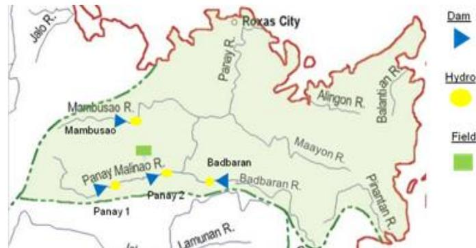
Figure 4: Panay River Basin with Proposed Facilities (Imaged adapted from Japan International Cooperation Agency (1985))
