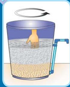
**4** Remove turbid water with a cup. Replace the basin and add more water. Repeat the stirring process for two additional times
