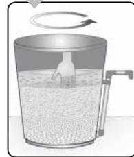
**4** Remove turbid water with a cup. Replace the basin and add more water. Repeat the stirring process for two additional times
