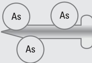
Arsenic (As) particles are effectively adsorbed on the rusted iron nails surface.
