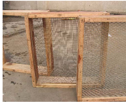
Use gauge 2 screen for gravel, gauge 5 for coarse sand, gauge 14 for fine sand
