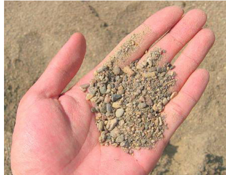
Poor coarse sand - non uniform size, mixed up with lots of dirt, silt, and fine sand
