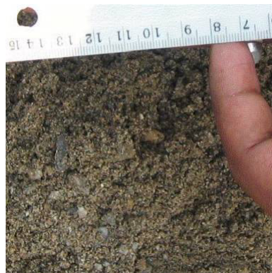
Poor fine sand - non uniform size, mixed up with lots of dirt, silt, and large particles
