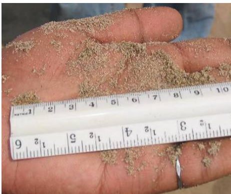
Ideal fine sand - uniform size, little dirt and silt, no large particles
