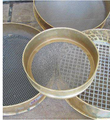
Mediocre quality sand/gravel can be improved by sieving
