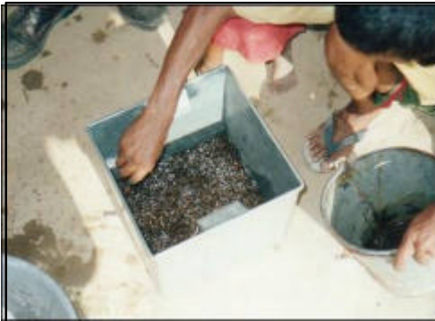
Placing iron nails into diffuser box
