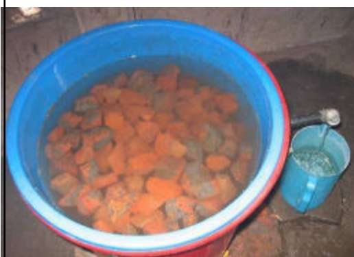
Top view of filter and basin with iron nails and brick chips
