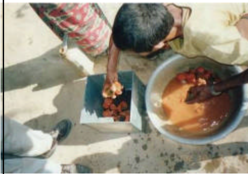
Placing brick chips into diffuser box
