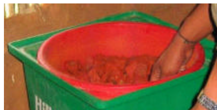
Placing brick chips in the diffuser box
