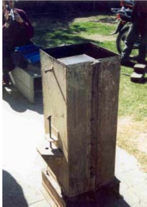
Figure 48 - Steel Mold for Concrete BSF Shell (assembled)
