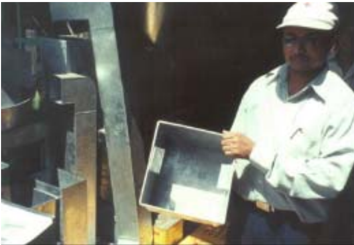
Figure 8 - A newly made Metal Diffuser Box from the Metal Workshop
