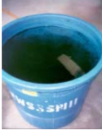
Figure 23 - ENPHO's Black Coagulation Powder Added to 20 L of Water
