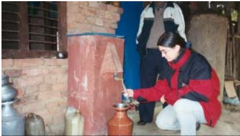
Figure 37 - Sophie Walewijk Measuring Flow Rate at Tek Bahadur Hamal's ABF in Devdaha VDC.
