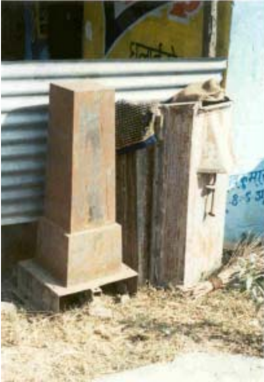
Figure 47 - Unassembled Steel Mold – Inner Mold (left) and Outer Mold (right).
