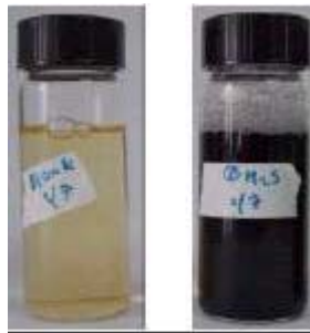
Figure 20 - P/A H 2 S Bacteria Test Showing Uncontaminated Sample (left) and Contaminated Sample (right)
