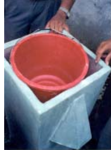
Figure 26 - Diffuser Bucket Replacing the Metal Box in the ABF
