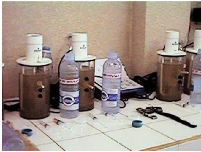
Figure B-4: Jar-testing equipment used on the field study
