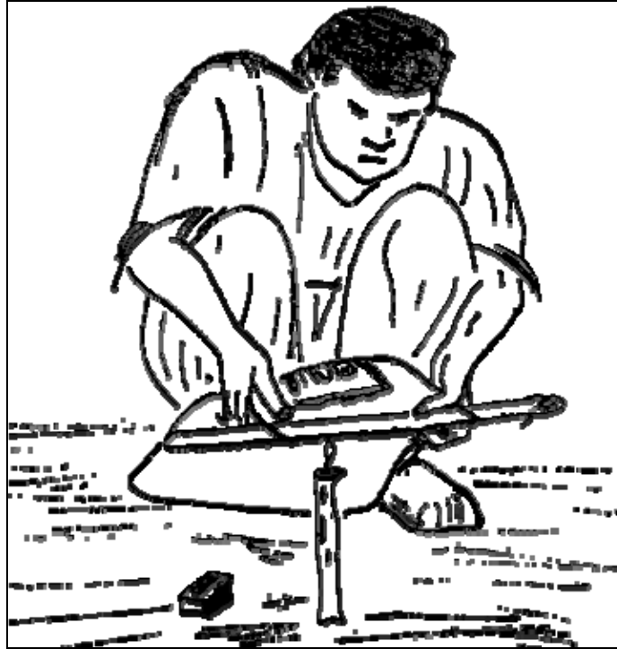
Figure 4.29 - Candle and hacksaw blade method of sealing plastic bags (FAO, 1994)
