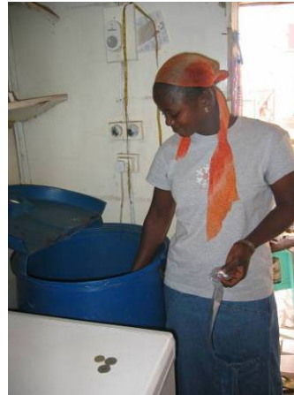
Figure 4.2 - Hand-tied sachet water being manually filled
