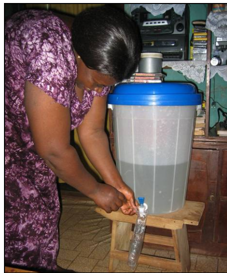
Figure 4.24 - Ceramic pot filter use in hand-tied sachet-water production
