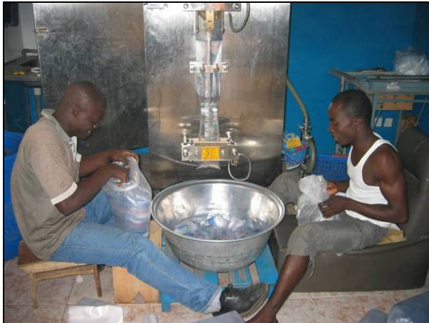
Figure 4.1- Factory-produced sachet with sealing machine in the background
