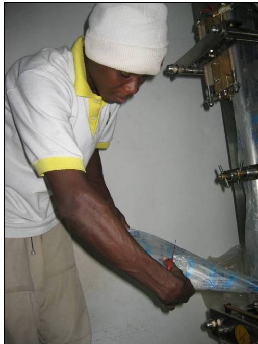
Figure 4.10 - Final adjustment of roll and trimming below seal
