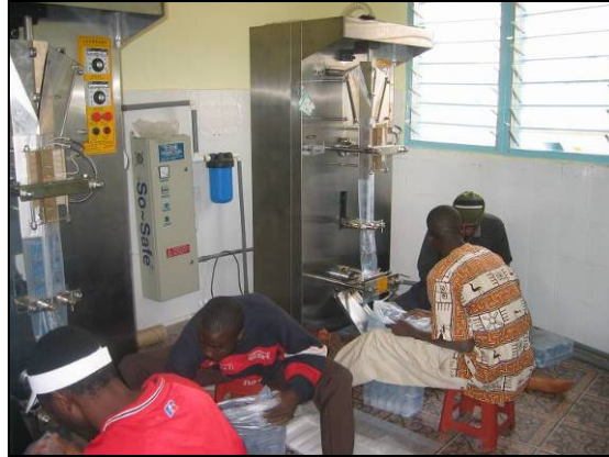
Figure 4.3 - Typical sachet-water factory set-up
