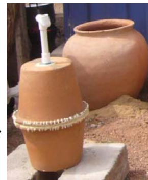
Figure 6-2 An Assembled KWK (without the siphon) in Front of the Ceramic Water Storage Vessel
