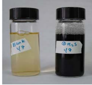
Figure 2-2 Negative (left) and Positive (right) Test Results
