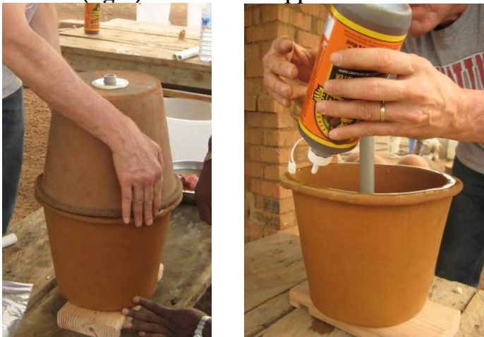
Figure 6-4 (left) Best Alignment Found to Match Up the CPFs (right) Gorilla Glue Applied to Rim
