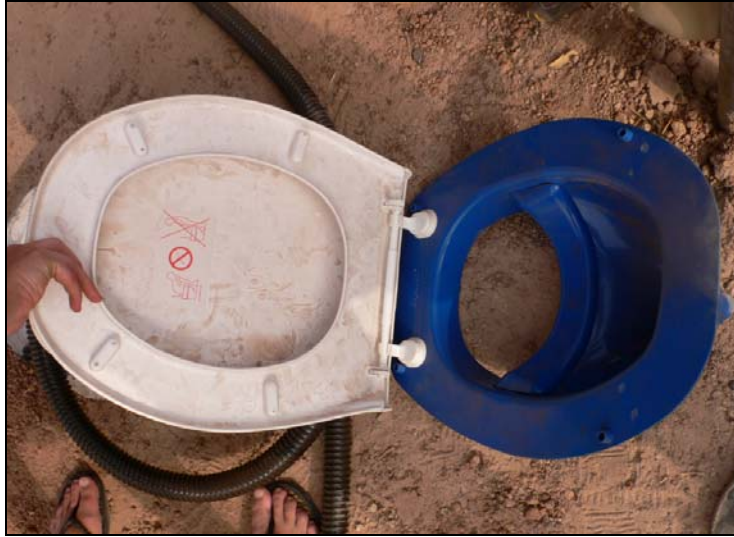
Figure 3-4 The type of urine-diverting seat used for the composting latrine
