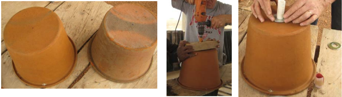
Figure 6-4 (left) Best Alignment Found to Match Up the CPFs (right) Gorilla Glue Applied to Rim
