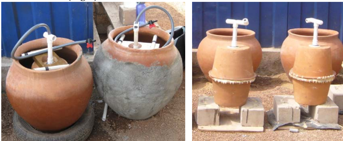
Figure 6-1 (left) Two KWK Installed in Water Vessels (Right) Two KWKs In Front of Their Water Vessels
