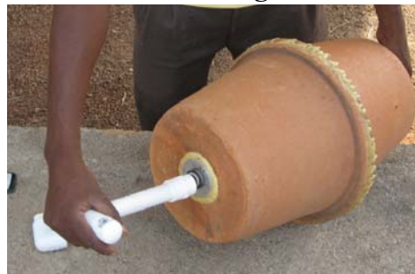
Figure 6-6 (top left) PVC Pipe With Holes Drilled In (bottom left) PVC Pipe Being Re-Threaded (right) Screwing in PVC Riser Pipe with O-Ring Seals
