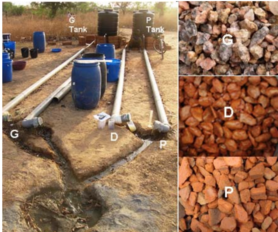
Figure 21 Pilot HRF media: granite gravel (G) left, local gravel (D) center, broken pottery (P) right
