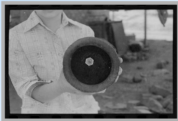
Close up of jam nut used to secure tap on inside of pot at Oriang
