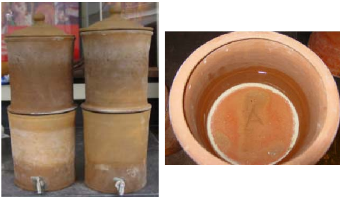
Figure 3: Terracotta Ceramic Filters Manufactured at Madhyapur Clay Crafts (Nepal, January 2002)
