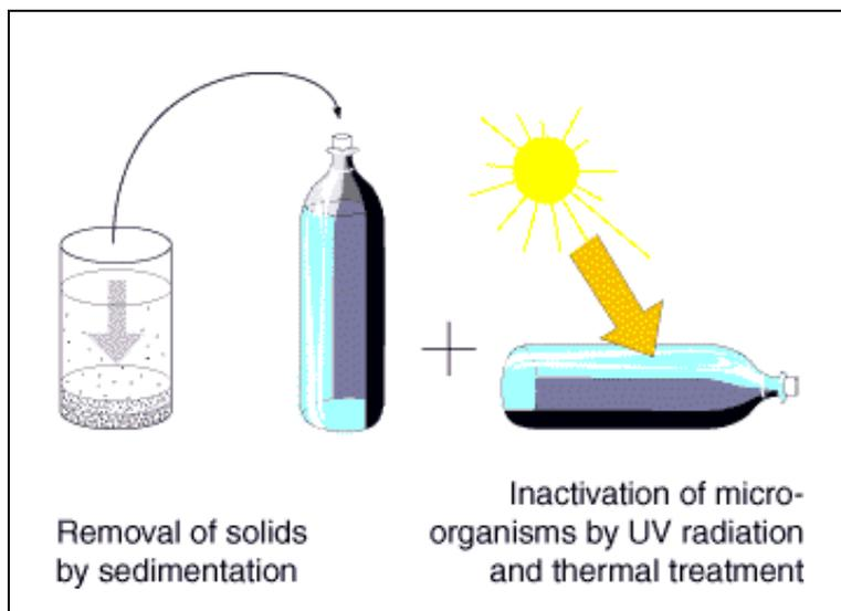
It is important that the bottle is in good condition since excessive scratching reduces that amount of light that can reach the water, which would reduce disinfection. It is also important that the water have a turbidity level below 30 NTU because the suspended particles scatter light, reducing the amount of light penetrating into the bottle. Additionally, half of the bottles can be painted black to increase light absorbance and hence increase the water temperature.
