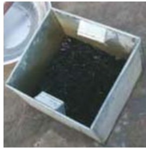
Diagram 2: The Concrete Arsenic Biosand Filter and the Metal Diffuser Basin Used for Nails
