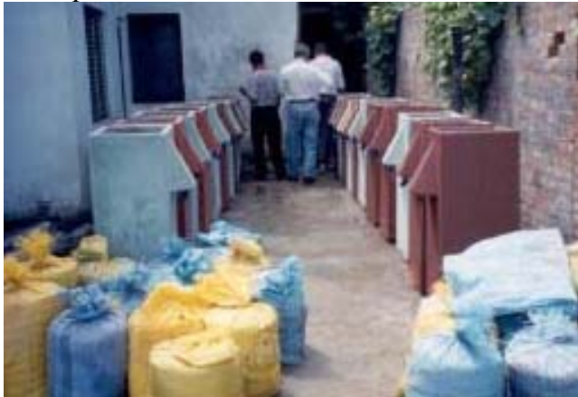
Mass production of concrete filters in a VDC
