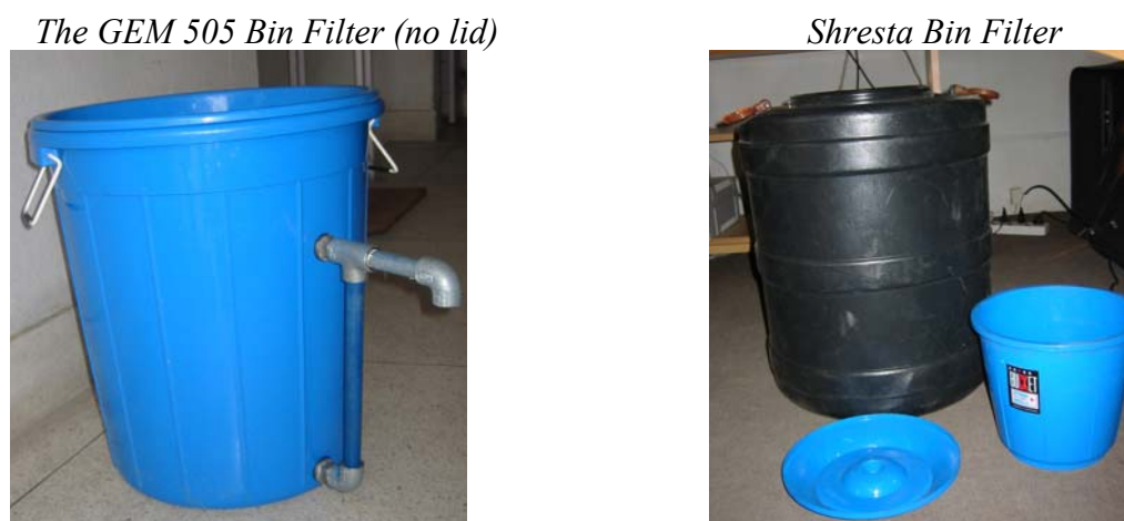
Diagram 4: Alternative ABF Designs with Locally Available Plastic Containers
