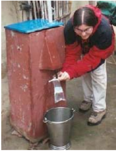
Diagram 2: The Concrete Arsenic Biosand Filter and the Metal Diffuser Basin Used for Nails
