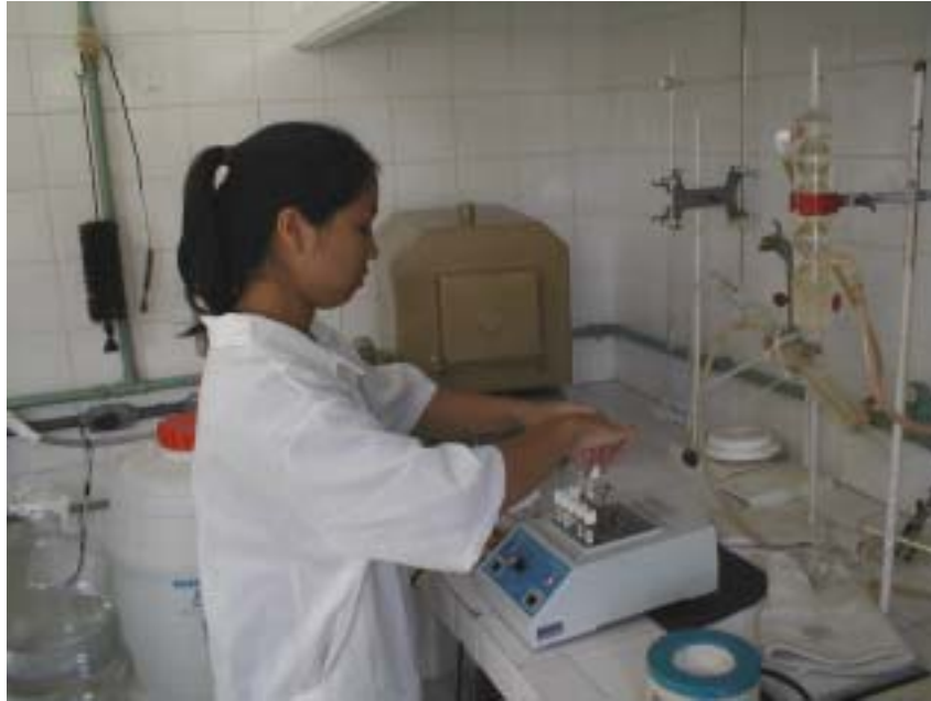
Figure 3-6 Sample Cooking in Hach COD Reactor
