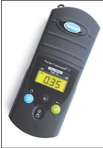
Figure 22: DPD Pocket Colorimeter II Test Unit (Hach 2008)
