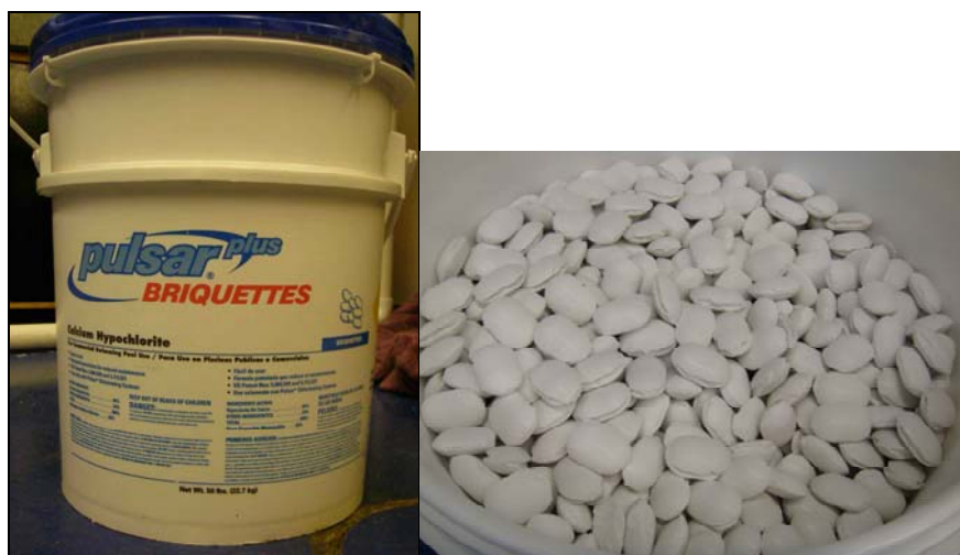
Figure 13: High-Test Hypochlorite (HTH) Container and Briquettes for Pulsar 1 System
