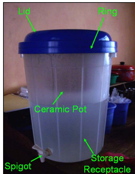
Figure 5: The Kosim Filter and its components (PFP, 2007).
