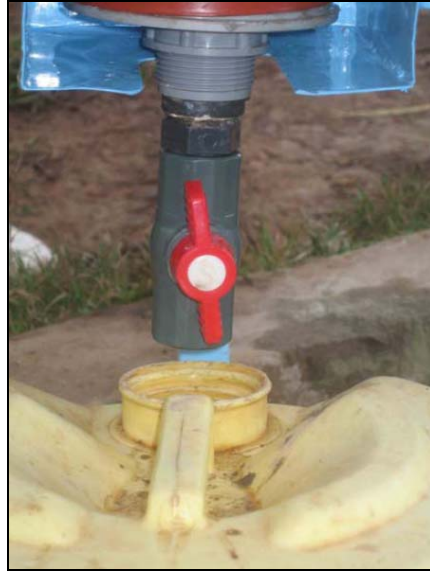
Figure 8: Close-Up of Chlorine Dispenser and Jerry Can (Berens and Van Dusen 2007)
