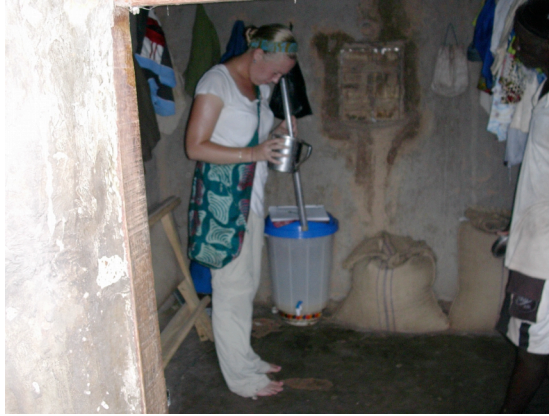
Figure 18: Measuring the turbidity of KOSIM filtered water (photo: Amin Hussein)
