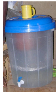
Figure 1: KOSIM ceramic water filter and safe storage unit (photo: author)
