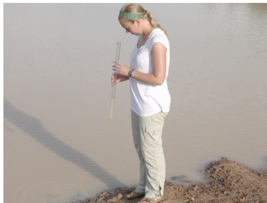
Figure 17: Measuring the turbidity of unfiltered water from a local source in Northern Region Ghana (photo: Amin Hussein)
